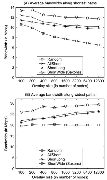
Figure 8: Overlay bandwidth.
