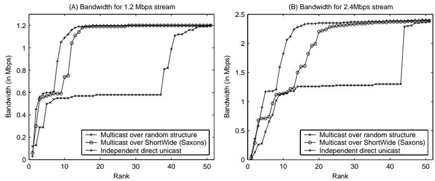
Figure 17: Multicast bandwidth on 52 PlanetLab sites.
