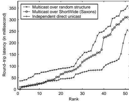
Figure 16: Multicast latency over 52 PlanetLab sites.
