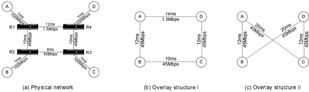
Figure 1: An example to illustrate overlay structure qualities.
