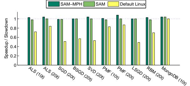
Figure 4: Performance of standalone applications using SAM-MPH, SAM, and default Linux on the 80-CPU Haswell. The performance metric is the execution time speedup (the higher the better) compared to that of the best static task→CPU mapping determined through offline testing.
